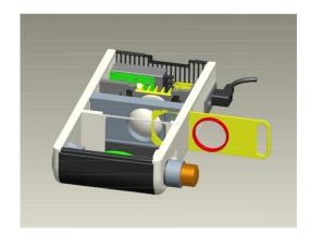
2. Pulling the filter slide all the way to the right (first detent) allows a color filter to be installed or removed. The color filter has very fine threads and must be GENTLY screwed into the opening on the front side of the filter slide. A light touch is required, as forcing the threads will result in permanent damage.
