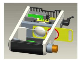
3. Pushing the filter slide to the left will then engage the second (middle) detent. This is the operating position with the color filter OUT of the light path.
