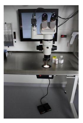
2. Increase brightness by pressing on the right pedal. Decrease brightness by pressing on the left pedal.
