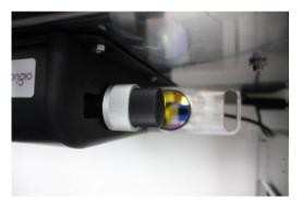
1. The TLB Light Source has the ability to switch one colored filter in or out of the light path. The handle for the filter slide is located on the right side of the TLB Light Source. It is stainless steel and located between the mirror control knob and the power cord. The filter slide can be pulled to the right and has three detents. It has a positive stop to prevent it from being pulled completely out of the base.
