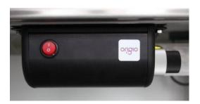
1. Turn the Light Source on by pressing the "I" (top) side of the red rocker switch, located on the front of the unit.
