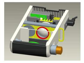
4. Pushing the filter slide further to the left will then engage the third detent. This is the operating position with the color filter IN the light path.
